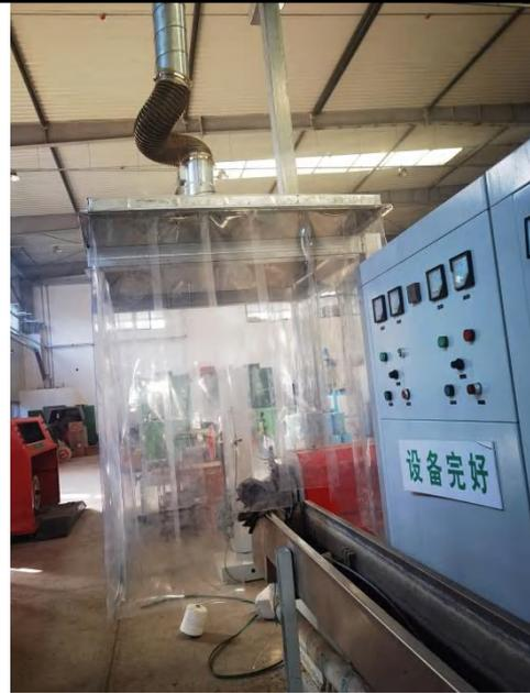
挤包护套挤出机-集气罩和软帘
